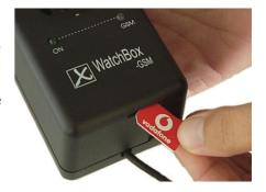
**ACHTUNG**: Before inserting/removing the SIM card ensure the **AlarmBox-GSM** is not connected to the power supply (i.e. pull out of the wall outlet), otherwise the complete contents of the SIM card, not only the contents of the phone book could be destroyed. In this instance the SIM card user will need to exchange the card with the provider, which will incur further costs.
